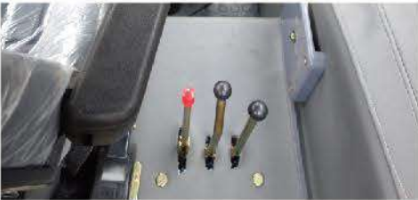
Equipped flat floor, hanging pedals, side manipulation. The use of 16F+8R shuttle shift transmission, it provides various gear selections, and makes a reasonable velocity distribution;
