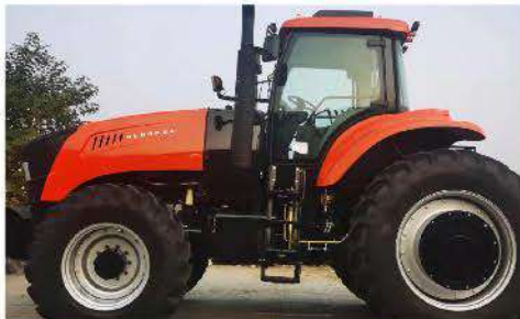
Shangchai six-cylinder engine, turbocharger, inter-cooling, 12 hours rated power: 221kw,
