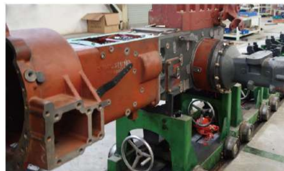
Testing of Gear Box
