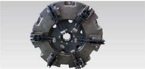
YTO brand independent-operation, dual-action clutch with reliable performance, large torque reserve coefficient, and high transmission capacity;
