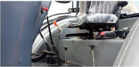
Hydraulic driving brake system and handle –manipulated stop braking system, high safety coefficient;
